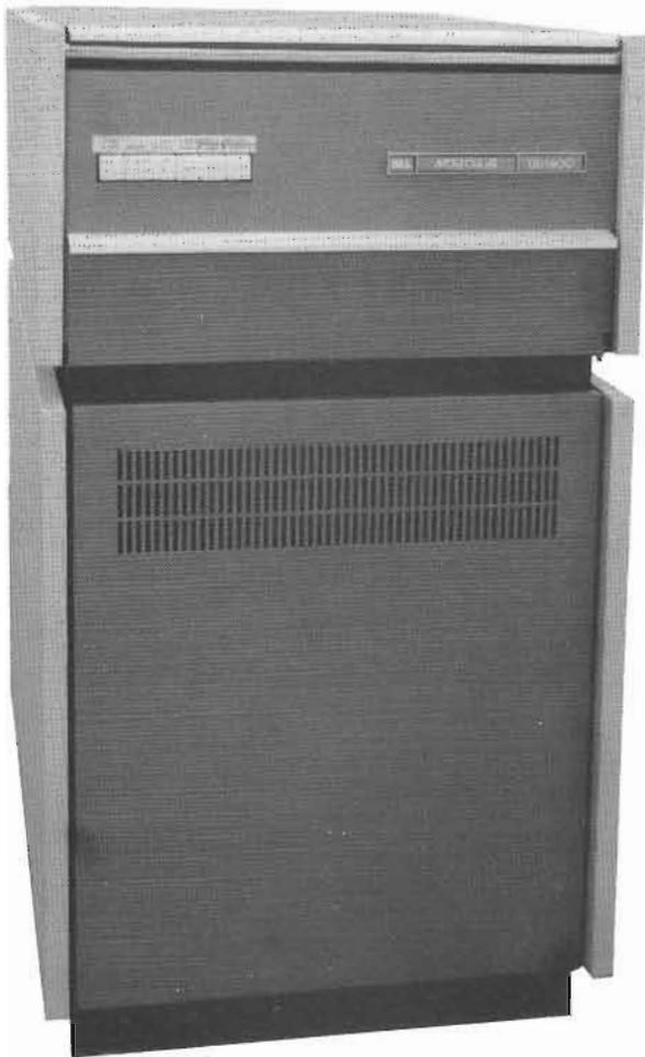
Electronic accounting and data processing require large files to be stored in such a way that they can be read and amended at high speeds without endangering the security of the information. The DD 1600 gives MOLECULAR the ability to store up to 6.4 megabytes (3.2 million words), or about ten million characters.
